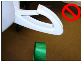
Figure 5 - Sling loop separated from the P-600 carry bar hook.
