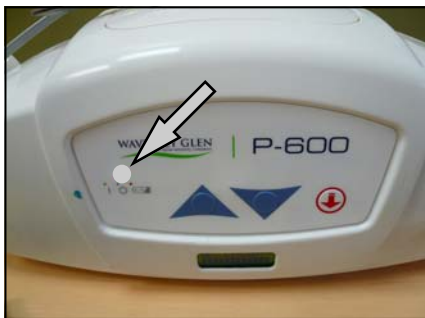
Figure 4B - The indicator light of the lift is normally off when not in use.
