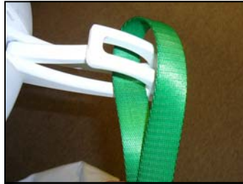
B) - During the preparation for the patient transfer, the sling loop flipped over.
